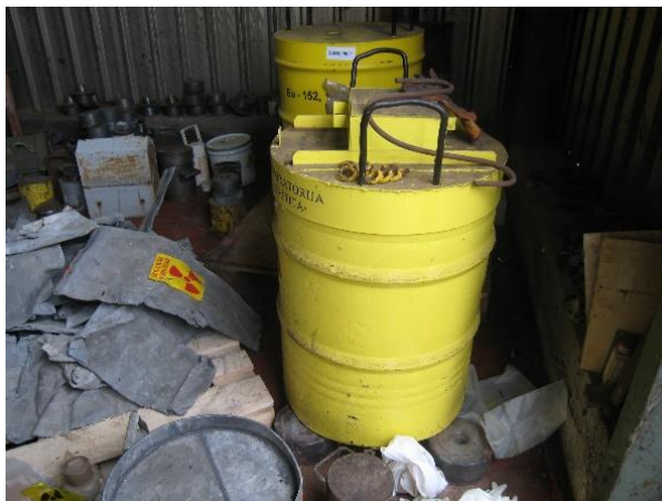
Figure 32. Shielded containers for storage of spent sealed sources from radioactive lightning rods
